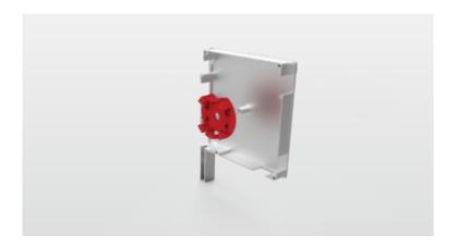
b) Drill holes in the side wall with a  $\emptyset$  3.5 mm drill bit using the motor mount as a template.
